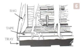
Pull the bag over the rolled edge of the tray for a distance of 1 1/2 inches. With the bag pulled over the rolled edge all the way around the tray, reach under the bag and gently pull protective backing off the tape. Press bag against exposed tape while continuing to remove the backing.
