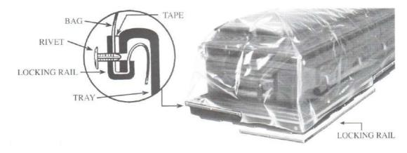
Reposition locking rails covering the bag at the rolled edge. Push rivets into the pre-drilled rail until rivet is flush with surface.
